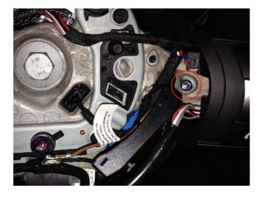
Step 5: Disassembly and assembly of paddle shifter
